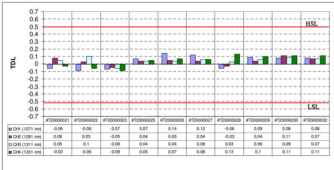
Fig:5 Typical TDL over temperature rage -5°C – 80°C (measurement data) (Temperature Dependent Loss)
